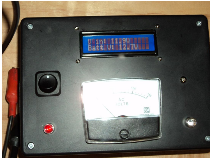
Figure 4.7: Inactive System Not Charging the Battery
