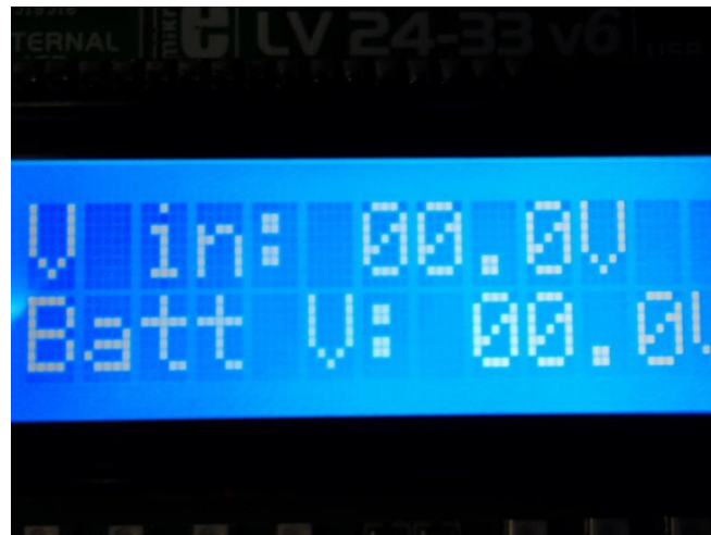
Figure 4.2: LCD Display of Grounded Inputs to the Microcontroller
