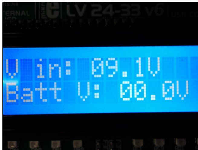
Figure 4.4: LCD Display of V in Measurement of a 9V Battery
