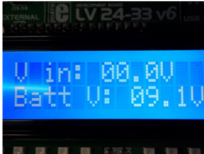
Figure 4.3: LCD Display of Batt V Measurement of a 9V Battery
