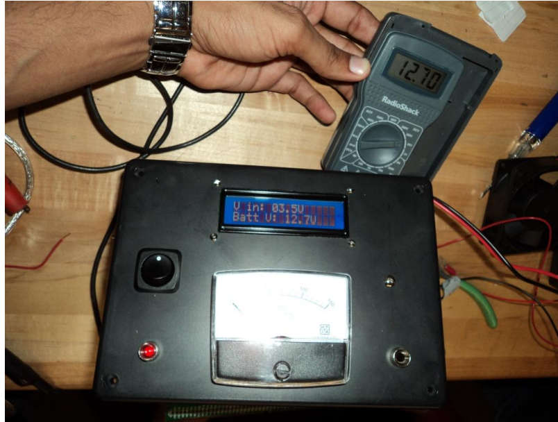
Figure 4.5: Confirmation of Battery Voltage Reading
