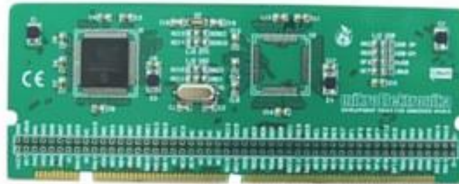
Figure 3.16: PIC24FJ96GA010 Mounted on an MCU Card
